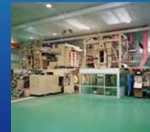
The world's only continuous vacuum metallizing machine
